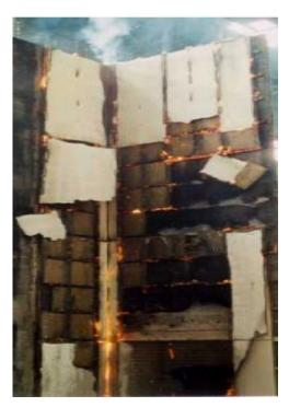
The duration of the fire load is 30 minutes. Test runs for 60 minutes
